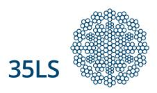
35LS is a conventional low rotation resistant rope consisting of three layers of strands the inner two layers spun in the opposite direction to the outer layer of strands manufactured in accordance with EN 12385.
